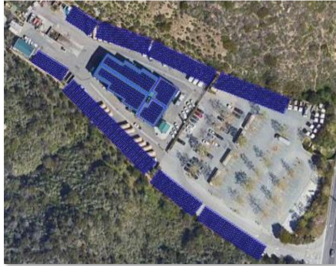
FIGURE 7: CORPORATION YARD HELIOSCOPE MAXIMUM PV SITE DESIGN
