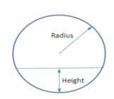
Square Ft of Half Full 24-in Pipe Where Radius = 1 ft Height of Water = 1 ft Area = 1.5708 sq ft 1.5708 sf x 4,500ft = 7,068 cu ft where 1cf = 7.48052 gallons
