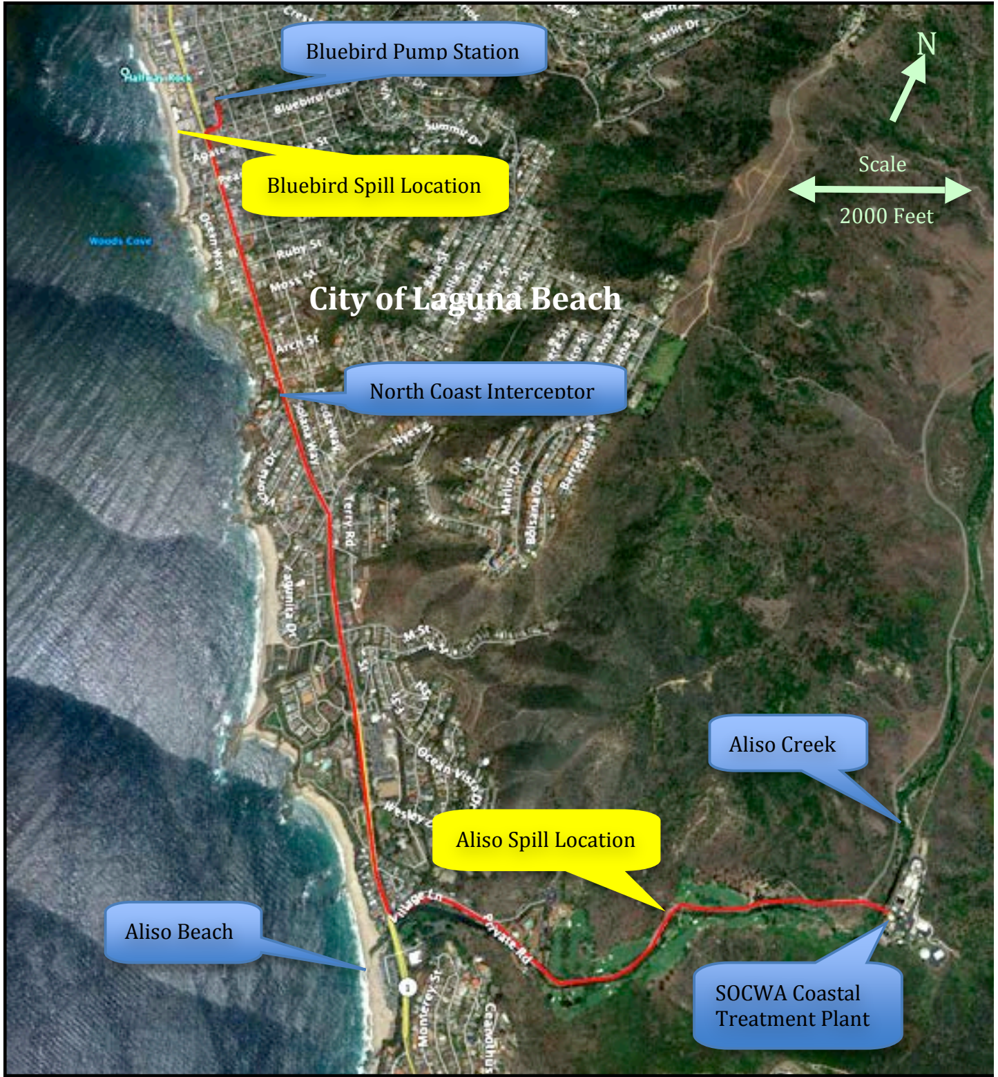
Figure 1. North Coast Interceptor sewer line, Aliso Creek, and spill locations.
